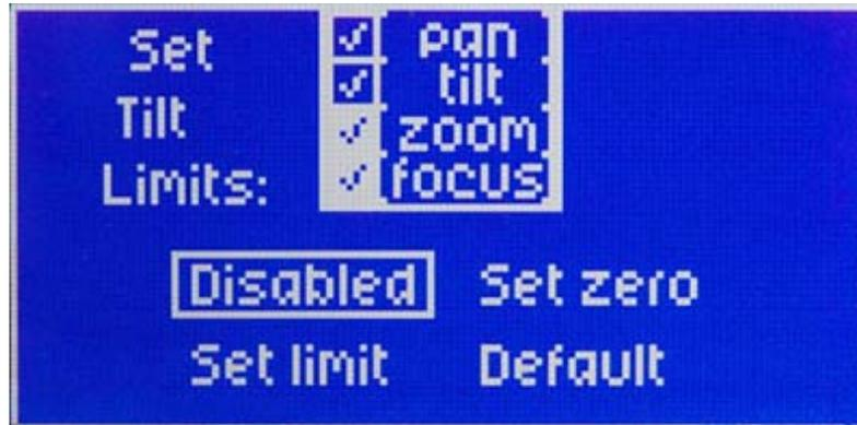
Press "Accept" to enter the Soft Limit menu. Then select the desired motor with and select knob (or +/- keys). Press "Accept" to enter the menu for that motor.
