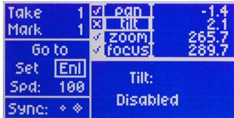
Press "Setup" on the Enable control to enter the Enable menu. Then select the desired motor with the select knob (or +/- keys). The left side of the motor display will show the selected motor's enable status. Toggle between enabled and disabled by pressing the "Accept" button. Place the motor in neutral by holding down the "Setup" button, then pressing the "Accept" button.
